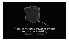
The brewer will automatically fill the internal hot water tank with water and then the water will be heated. This will take about three minutes. During the heating period, "Brewer is heating" will be displayed on the touch screen.
