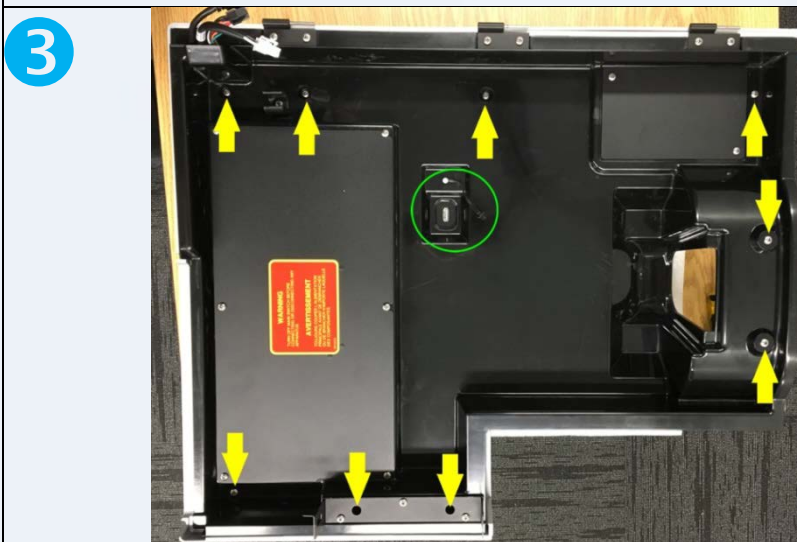
3 Disconnect the plug from the USB port and remove the nine screws securing the inner door to the outer door.
