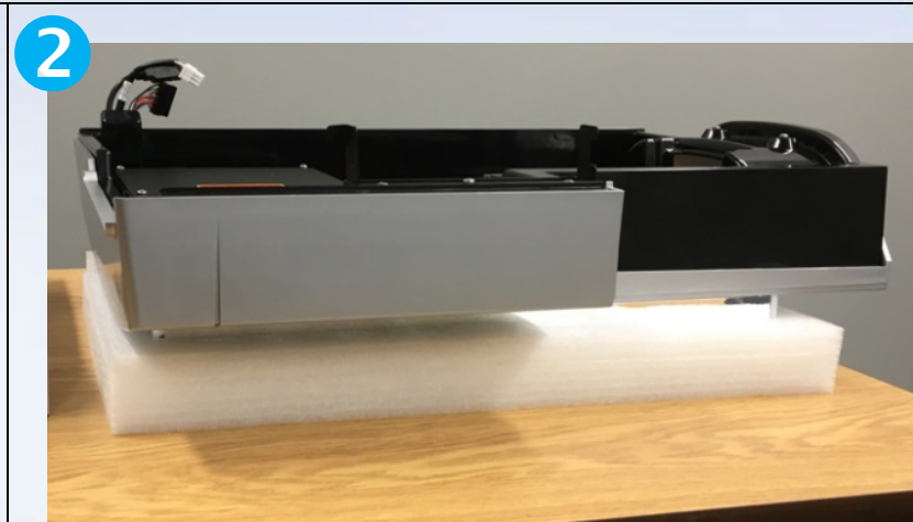
2 Lay the door (with the protective foam) flat on a table.
